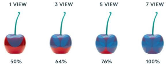
The Total View system analyzes more of the cherry's surface. It also removes false positives which can be caused by the cherry's stem being classified as a defect.
