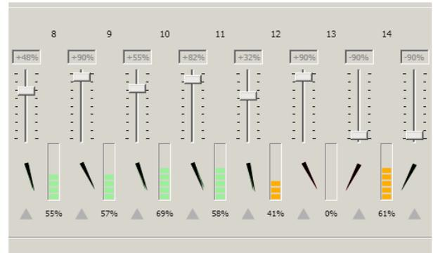
The Compac Dynamic Lane Balancing interface maintains an even flow of cherries across all lanes for maximum efficiency. The system also lets operators monitor the real-time status of the system and alerts them to potential problems.
